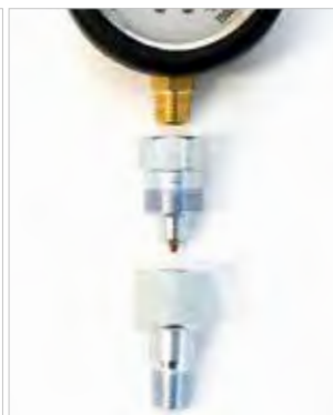
CP 210 coupling for pressure gauge - gaugebracket. Allows you to remove the gauge from the bracket. Reduces the risk for damage if such transportation. Thread: 1/4" NPT.
